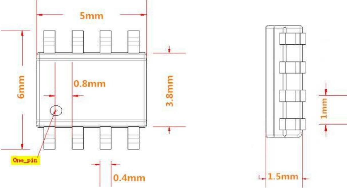
Unless otherwise prompted, all the sizes are marked as: (mm), tolerance:  $\pm 0.09\text{mm}$
